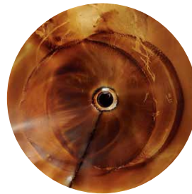
ISO VG 46 Mineral Hydraulic Oil: result after 1,000 hours (actual initial failure at 500 hours)
