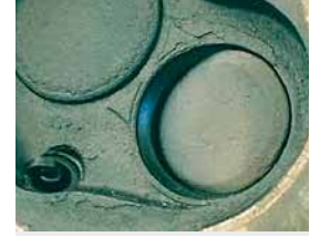
Figure 8 A recessed valve
