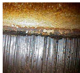
Figure 1 A defected anti-polishing area on liner
