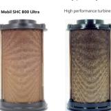
**Mobil SHC 800 Ultra** shows improved deposit control over high performance turbine oil.
