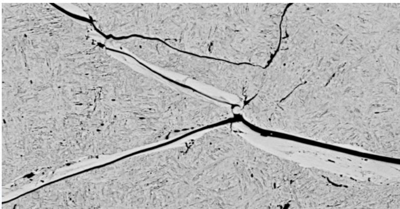
Around 60% of the industry's high speed bearing failures are caused by white etching cracking
